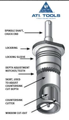
**NOTE:** Skirt remains stationary when in contact with the cutting surface, enabling the operator to view the cutter.
