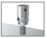
Recently, ATI developed a Hi-Lok® removal socket that has internal teeth that bite into the collar material. Using a Hi-Lok® ratchet or Hi-Lok® Roller Clutch Wrench, the operator places the socket over the collar and turns the ratchet. The socket's teeth dig into the collarmaterial with sufficient force to gain a hold of the collar so that it can be unscrewed. Again, a hex wrench may be used to stop the pin from rotating as needed.
